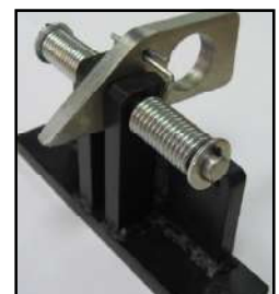
Lock security system, track and pin details.
