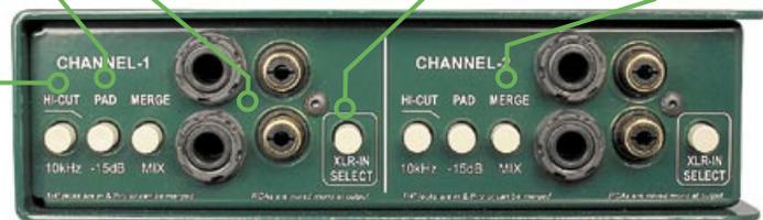
**+4dB XLR INPUT** for balanced line-level sources like mixing consoles and pro VTRs.
